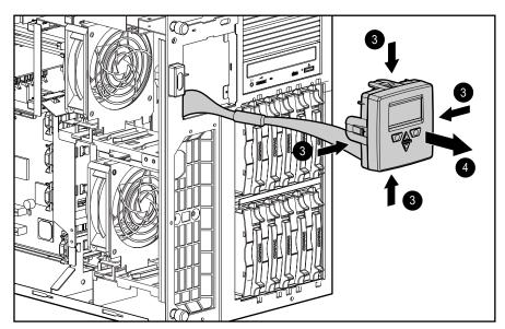
Figure 2-10. Removing the Integrated Management Display
